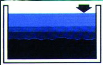
**Settle:** One of the major advantages of the SBR system is the creation of “perfect” conditions for the **Settle** period. There is no inflow of waste, no mixing and no injection of air. A healthy activated sludge floc settles rapidly — in 15-20 minutes. A design time of one hour is most adequate for the **Settle** period.
