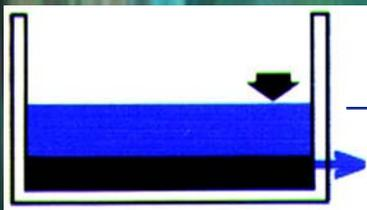
**Idle:** The **Idle** period is not a designated time frame but rather is that period between completion of **Decant** and the beginning of **Fill**. **Idle** periods occur when actual flows are less than design flows. When **Idle** periods are long, aeration is required to prevent septic conditions from forming.
