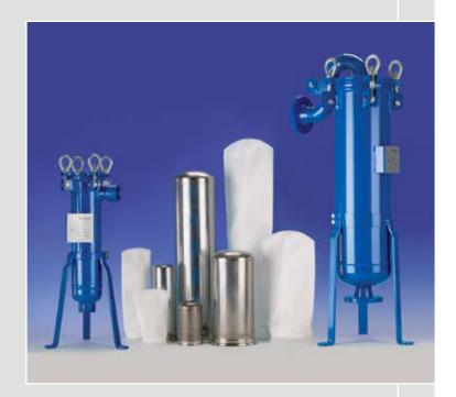
The goal of sizing a filter housing is to achieve minimal pressure loss ( $\Delta P$ ) across the clean filter—while balancing process effluent cleanliness, maintenance and bag change-out requirements.
